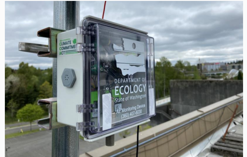
Ecology's custom-built SensWA PM 2.5 sensor
