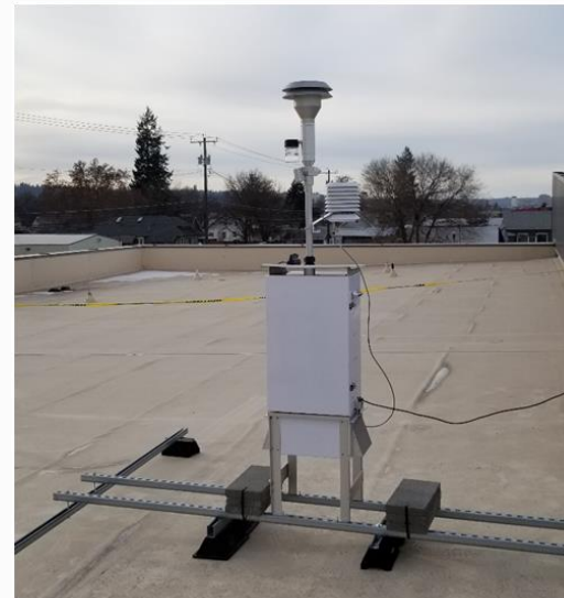
Ecology's custom-built SensWA PM 2.5 sensor
